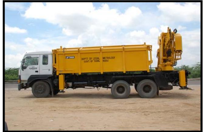
Observe above, the crane in transport position, where it is folded within 1.5m lateral space of the chassis, with outriggers flushed within body width of vehicle. Notice the in-line boom geometry, where the crane booms fold in between the twin columns over the slew
