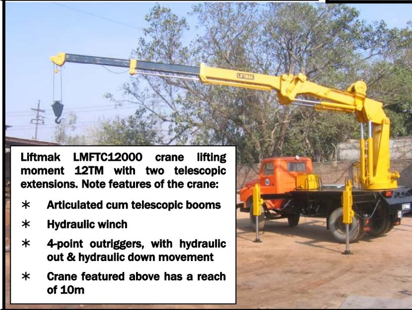
**Liftmak LMFTC12000 crane lifting moment 12TM with two telescopic extensions. Note features of the crane:**
