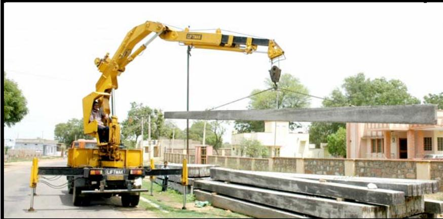
**Liftmak LMFTC8000 truck mounted hydraulic foldable crane handling poles**
