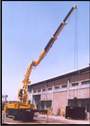
This photograph shows foldable crane with off-set boom geometry. This has the following drawbacks -
