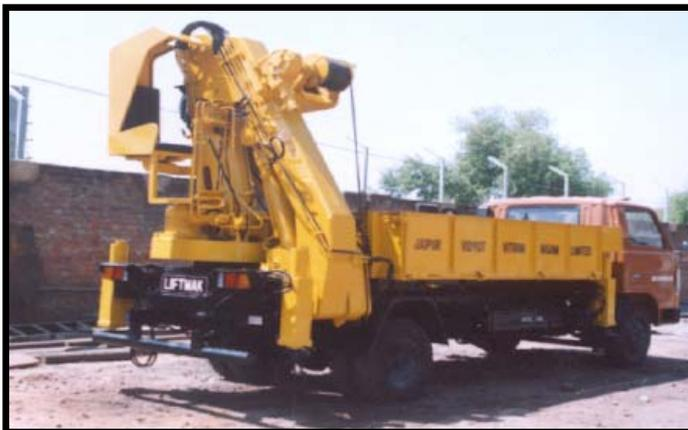
**Above:** Crane in folded position. Note that crane takes only 1.55m lateral space of chassis for mounting, leaving adequate space on truck body for 'self-loading'
