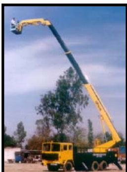
Telescopic cum articulated zero elbow design with basket resting on vehicle deck in stowed position for quick start up
