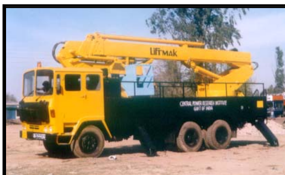
Telescopic cum articulated zero elbow design with basket resting on vehicle deck in stowed position for quick start up
