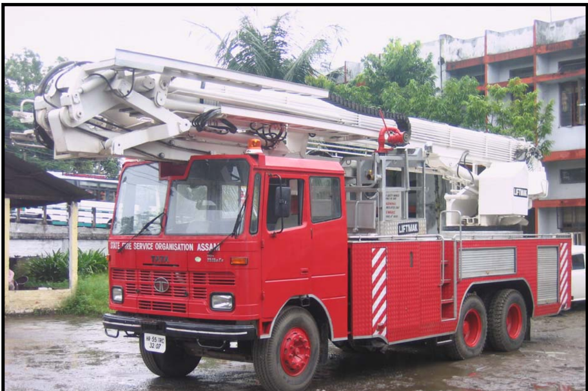
PICTURE SHOWS LIFTMAK 25M FIRE PLATFORM (SIMILAR DESIGN AS LMTHP32) IN STOWED POSITION. NOTE COMPACT STOWED LENGTH AND EASY ENTRY INTO CAGE FROM CHASSIS DECK FOR QUICK STARTUP
