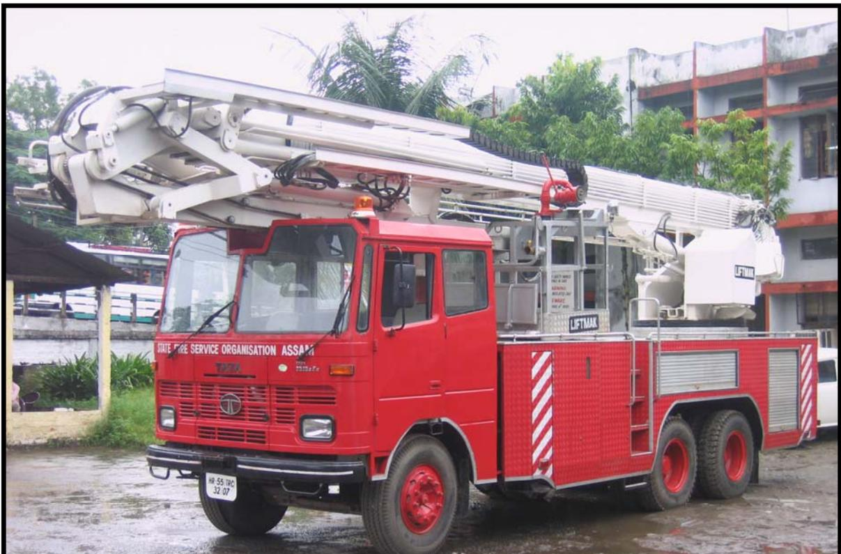
**PICTURE SHOWS LIFTMAK 25M FIRE PLATFORM (SIMILAR DESIGN AS LMTHP25) IN STOWED POSITION. NOTE COMPACT STOWED LENGTH AND EASY ENTRY INTO CAGE FROM CHASSIS DECK FOR QUICK STARTUP**
